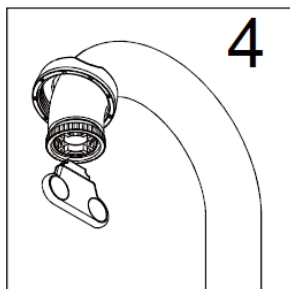
4. Take the wrench in the conversion & connection accessory kit to screw the thread coupling into water faucet.
