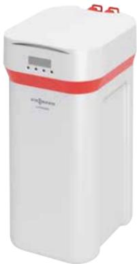
Viessmann water softeners work through a process called ion exchange which eliminates minerals like calcium and magnesium from the water. Resin neutralizes the minerals. Given its smooth surface, it makes water softeners run efficiently for a long time. Adding salt to the purifier enables the regeneration of resin – minerals are flushed away with waste water.
